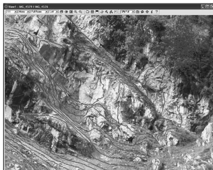
Fig. 4. DEM contour levels (projected in the XZ plane) from TLS data plotted on a stereoscopic model from a digital reflex camera (Socet Set Digital Photogrammetric Workstation). Noise in the TLS DEM is clearly visible in vegetation while contour levels fit properly in terrain.
